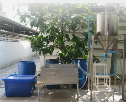
Constructed wetland for treatment of diethylene glycol contaminated wastewater by Burhead plant
